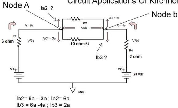
$$V_{ab} = I_{a3} - I_{b3} = 3a - 2a = 1a$$
