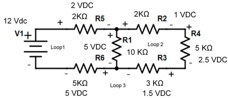
$$\text{Loop 1: } 2 \text{ Vdc} + 5 \text{ Vdc} + 5 \text{ Vdc} + (-12 \text{ Vdc}) = 0 \text{ Vdc}$$
