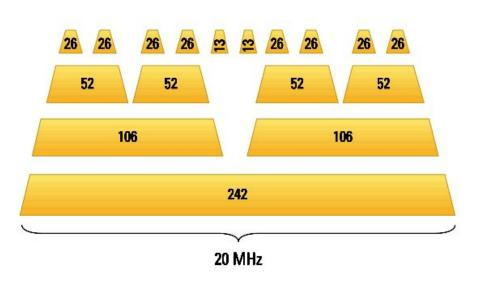
26, 52, 106, and 242 subcarrier RUs are designated to an 802.11ax AP when 20 MHz channel is subdivided, which roughly equates to 2 MHz, 4 MHz, 8 MHz, and 20 MHz channels, respectively.
