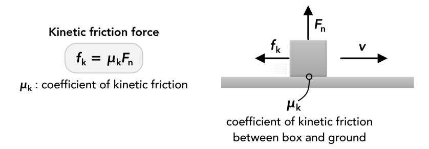
Example: A 10 kg box is sliding along the ground. The normal force between the box and the ground is equal to the weight force, 98 N. The coefficient of kinetic friction between the box and the ground is 0.4. The kinetic friction force is 39.2 N regardless of the velocity and any other horizontal forces.
