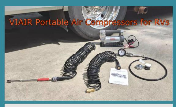
I think most RV owners understand the importance of maintaining proper tire inflation pressure. The problem is, if you wait until you're on the road to check tire pressure the tires are too hot for correct evaluation. Checking the inflation pressure when you stop to refuel doesn't make sense either; you will get higher pressure readings and if you let air out the tires they are under-inflated when they are cold again.
