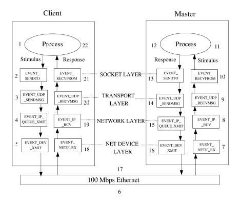
Figure 1: Linux Network Stack Instrumentation Points
