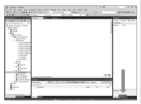
Expand the Lamps/Switches/Bitmaps collection in the toolbox and drag a Dip Switch element into the canvas.
