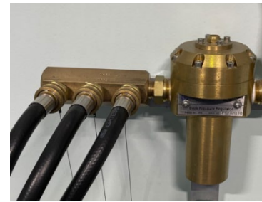
BIBS exhaust ports with back-pressure regulator
