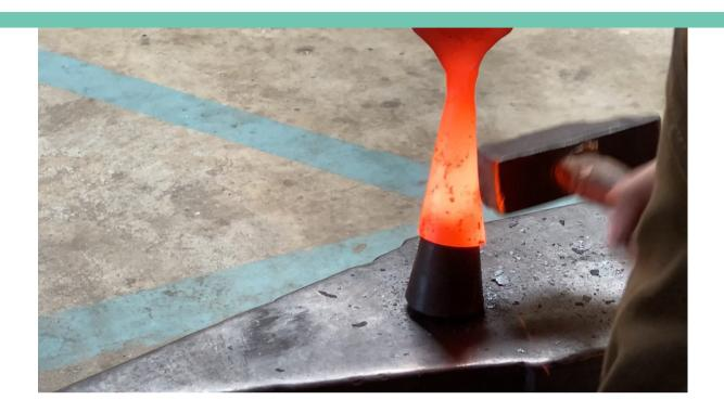
Clean and true up your cone with a cone mandrel. Hammer with a light touch and rotate while working.
