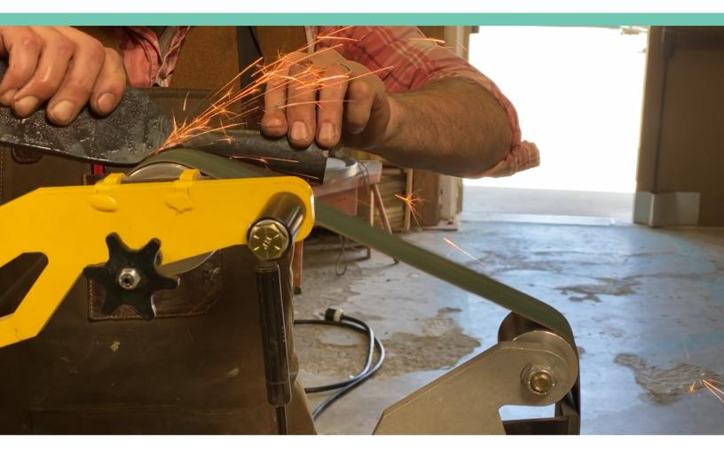
Dress and clean your forging by grinding or filing to final shape. I like to do a little grinding on the neck and shoulders so that the transition from blade to socket looks nice and clean. At this time I also grind or cut the end of the socket so that it is flat and true to the edges on the chisel.
