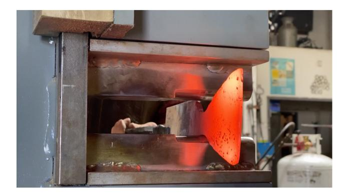
The fourth step is to finish fullering the neck to actual size. For a two inch wide chisel I leave 3/4". Use whatever method you used in step 1.
