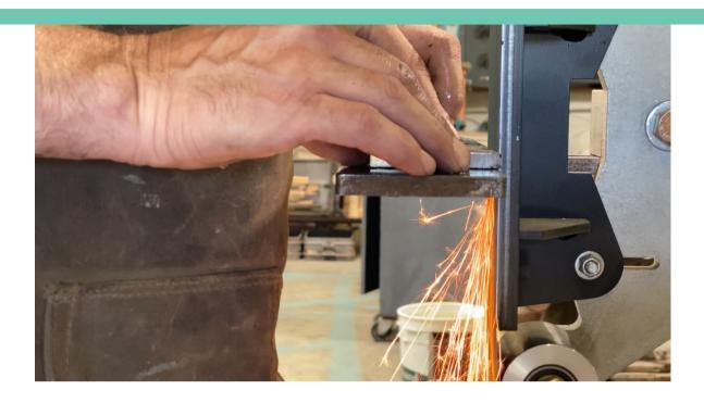
With a file, angle grinder or belt grinder squaure off the edges and end of the chisel. Then file or grind the bevel. Wood chisels have anywhere from a 25 to a 30 degree angle. The bevel angle depends on the work you wish the chisel to perform and the types of wood you will want it to cut. The harder the wood and the more abuse you expect it to take, the closer to 25 degrees your angle should be.
