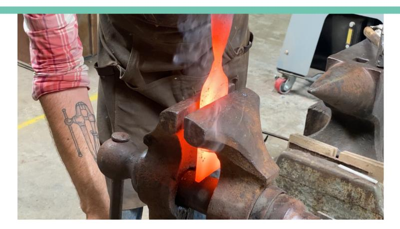
If your socket eye chisel is a Timber Frame Slick like the one I created in the video, it will need to have a curve in the handle or blade to give your hands room to hold the chisel while working. I begin the curve in the last third of the blade and continue it into the neck of the socket. Keep the socket straight so that you can fit the handle later.
