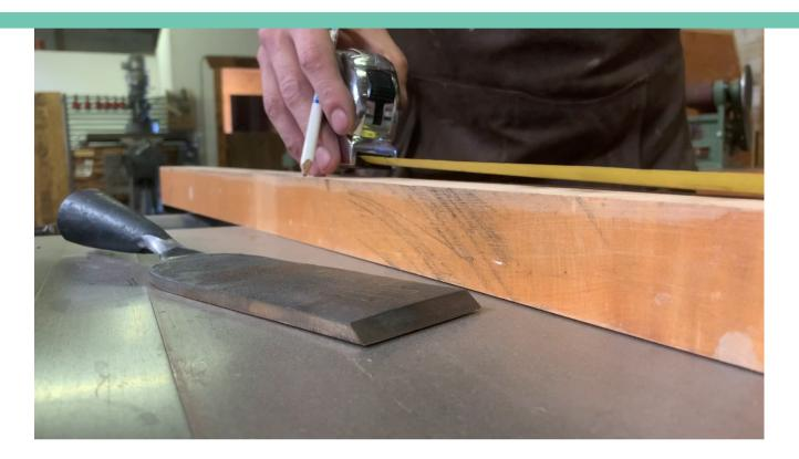
Time to make a handle. For the timber frame slick I have put an 18" handle on it including the socket. This gives me about 16" of finished handle to work with. You can use a wood lath or carving axe, drawknife or files to form your handle. Consider how you want to use the handle. I like to round the end so that it fits well in my palm and I carve in a neck and shoulders toward the socket end for my left hand. I find it ergonomical and easier to use this way.
