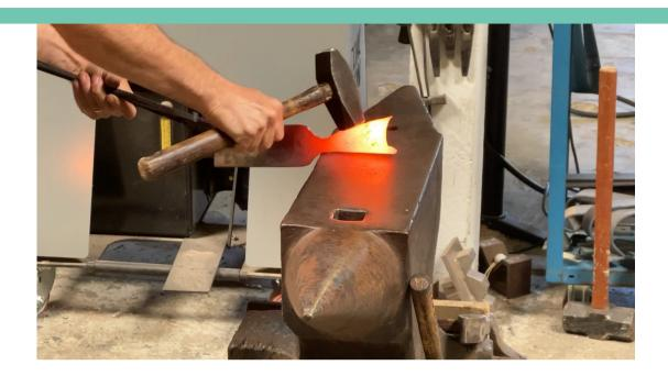
Finish rolling the cone into shape by lightly hammering and rotating your tongs 360 degrees. Be careful not to hammer with a heavy hand or you will flatten the work instead of creating a conical shape.
