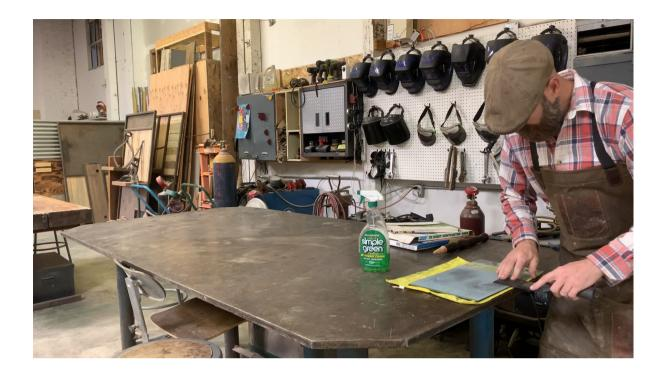
It is now time to make a usable tool by sharpening and setting the handle. Follow the steps in the sharpening video. I use epoxy to set the handle. Be sure to dry fit the hadle before glueing it in place. Don't add the glue until your fit and finish is satisfatcory.
