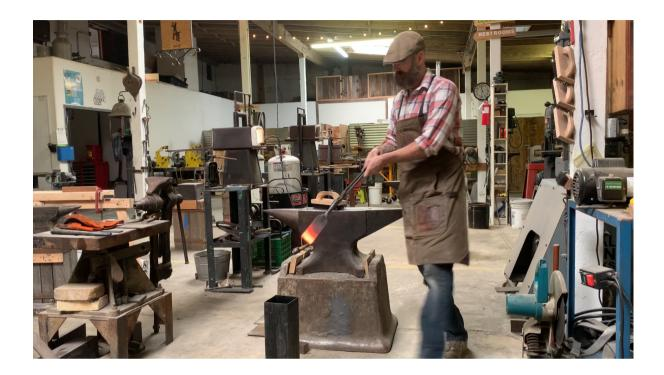
Quenching time. I used 5160 steel so I am quenching in oil. I do not want the entire chisel to be hardened material so I have only heated half of the blade. Submerge the entire chisel in the oil and gently stir until the heat has discipated. You can tell if it has cooled enough if it is no longer smoking when you pull it from the quench. Be prepared to temper as soon as you can.
