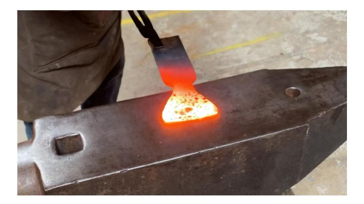
It is time to clean up your forging. I use a flatter. If you do not have one use gentle blows with the flat face of your hammer. The goal is to remove irregularities and unwanted hammer marks. Be sure that you have an even 1/8" thickness with tapered edges on the sides but not the top. I left room to grind the top of the cone which is why I am ok that the edges are a little rounded. They will get cut off anyway.
