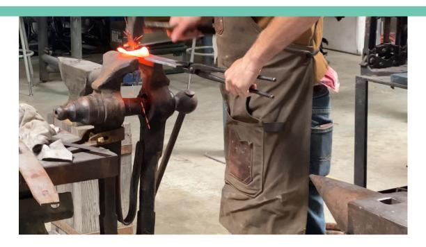
I begin to roll the cone using my hammer and two other points of contact. I like to use my vice and adjust the jaws so that the trangle has half an inch of contact on either side. Use the peen of your hammer and gently strike the middle until it has slipped free of the vice. Move to the anvil and continue to roll by hammering the edges down. Rotate while hammering so that you roll the cone instead of creating a taco.
