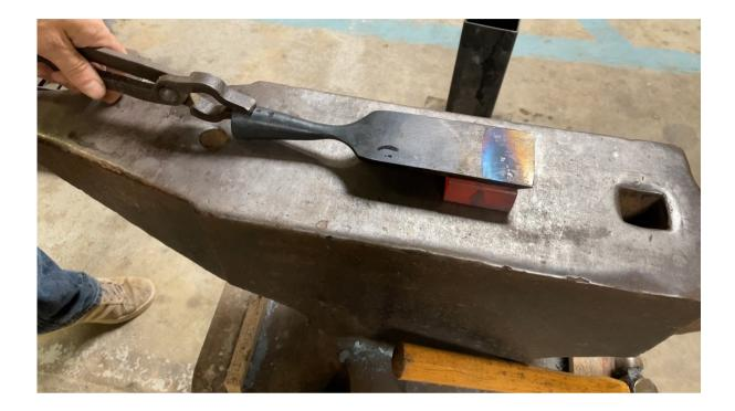
After quenching I sand the back of the chisel just enough so that it is reflective. During the heat for the quench I also prep a block of scrap steel and use it as a heat source to run colors. Be sure that the cutting edge of the chisel is off of the heat block so that you don't temper to soft. Allow the colors to run from the middle of the blade outward. As soon as I see straw yellow reach the cutting edge I quench in oil to hold the tempering treatment.
