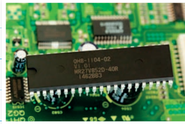
In a PC, the sets of instructions needed for the computer to start up are stored in ROM. These instructions need to be stored and saved even after the power is turned off.
