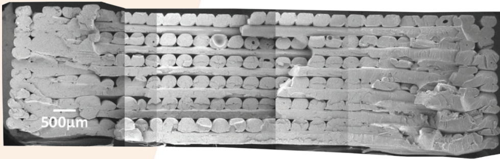
Figure 5.2: Electron microscopy image of a sectioned 100% infill 3D printed part using FFF technology. The darkened areas are gaps (voids). Using the scale bar on the bottom left, gaps as large as 20 \mu\text{m} can be seen forming during the deposition process. Additionally, the layer-by-layer structure (visible in grey) informs us about the extrusion pattern and the size of the nozzle (400 \mu\text{m} ). ©Gorski et al., A.I.S.C. (2015) p403-413
