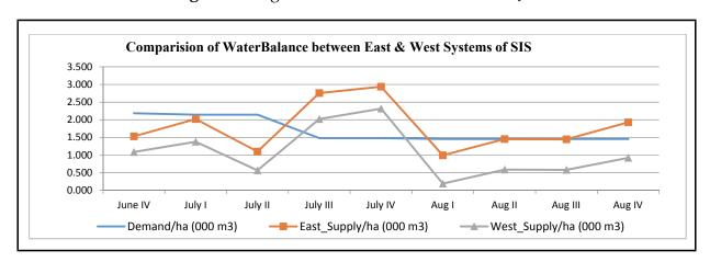
Figure 7: Comparison of water balance between East & West subsystems of SIS
