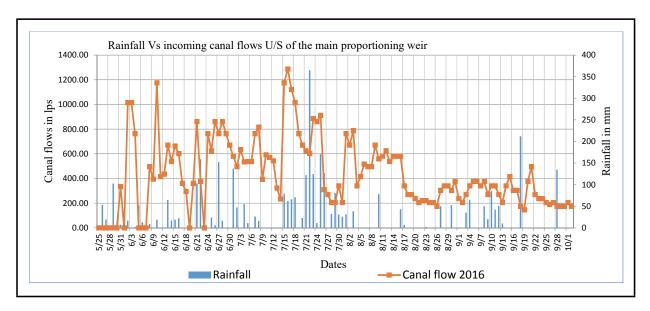
Figure 1: Rainfall vs main canal flows of JIS
