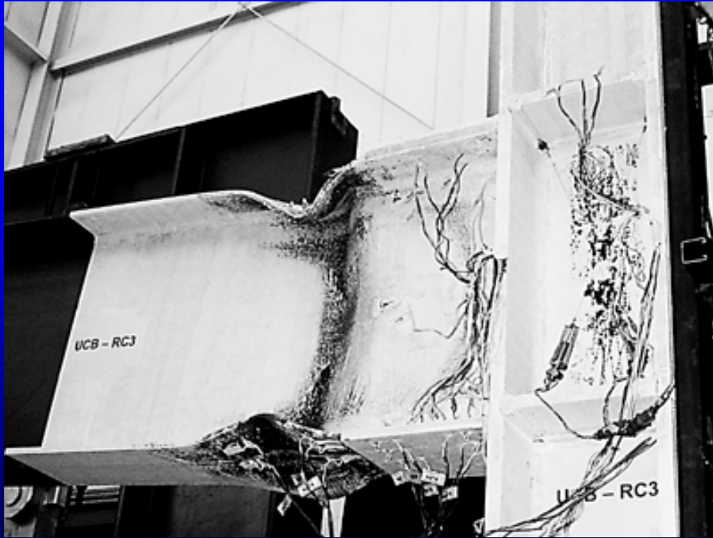
Local flange and web buckling
