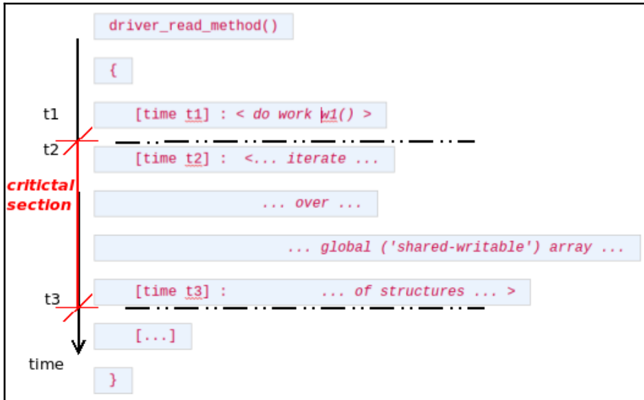
Figure 6.5 – Pseudocode – a critical section within a (fictional) driver's read method; it's wrong as there's no locking
