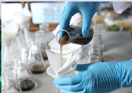
Decanting a solid-liquid mixture
