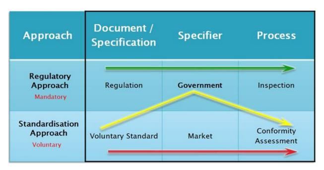
The green line at the top shows how a government develops a regulation, then specifies its use, and finally enforces it through inspection. An example is the current laboratory-licensing program used by the US FDA.
