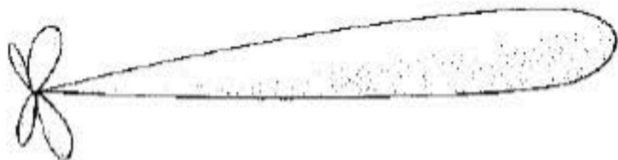
Figure 1303a. Freespace radiation pattern.
