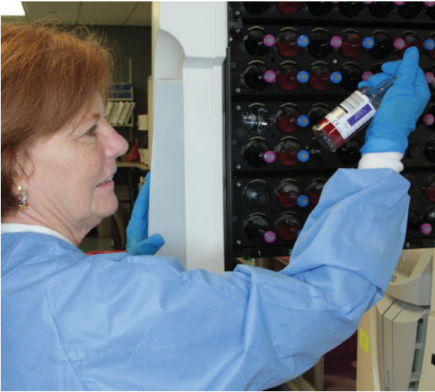
Figure 1-13 A microbiologist reviews blood cultures processed by the BD BACTEC™ FX blood culture instrument.
