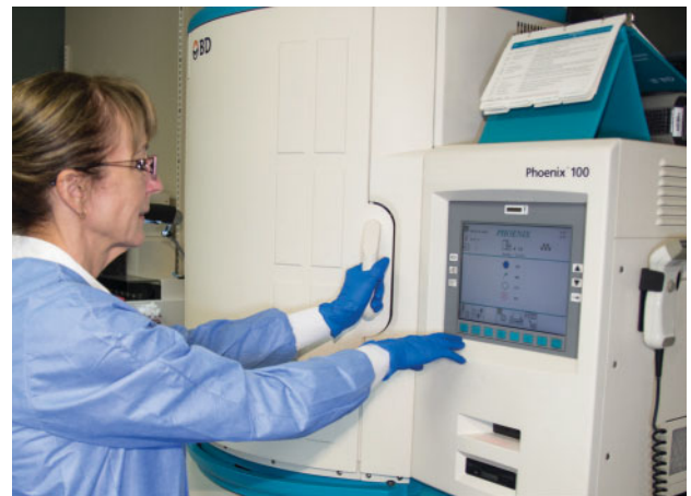
Figure 1-12 A microbiologist checks computer read out for antibiotic sensitivities from the BD Phoenix™ automated microbiology system.
