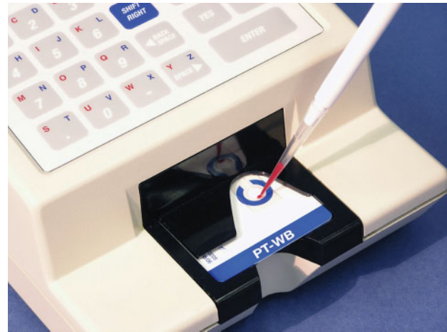
Figure 11-17 Whole-blood sample being added to the Cascade® POC barcoded assay card. (Courtesy Helena, Beaumont, TX.)
