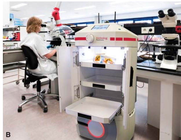
Figure 12-12 Robot specimen transportation system called the RoboCourier® Autonomous Mobile Robot. A: RoboCourier® in a lab after delivering a specimen. B: A RoboCourier® traveling down a hallway. (Courtesy Swisslog Healthcare Solutions North America, Denver, CO.)
