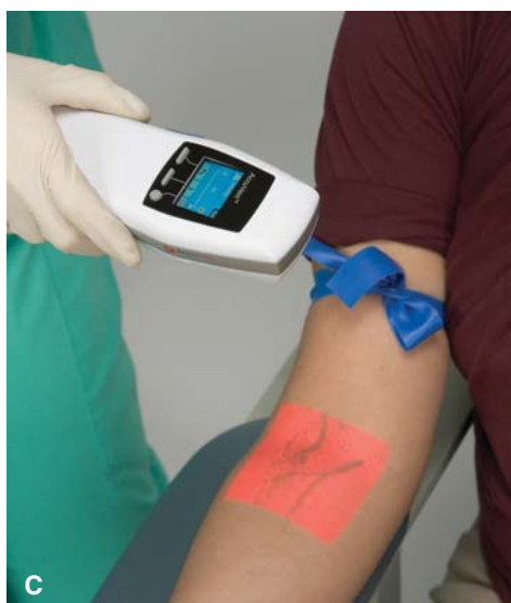
Figure 7-9 A: A Venoscope II transilluminator device. B: A vein appears as a dark line between the light-emitting arms of the Venoscope II. (Venoscope II, LLC, Lafayette, LA.) C: AccuVein AV300 being used to locate veins on a patient's arm. (AccuVein LLC, Huntington, NY.)
