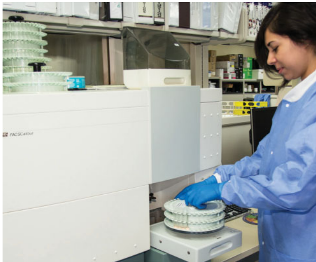
Figure 1-15 Medical Laboratory Scientist loads BD FACSCalibur™ modular analyzer with tissue samples for HLA testing.
