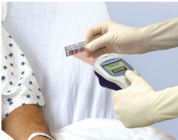
Figure 11-27 The PXP scanning a test strip barcode at the bedside. (Courtesy of Abbott Diabetes Care, Alameda, CA.)
