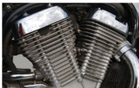
Figure 2 Motorcycle engine fins
