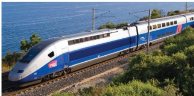
Figure 1 The French TGV (Train à grande vitesse) electric train can reach speeds of more than 500 km/hour
