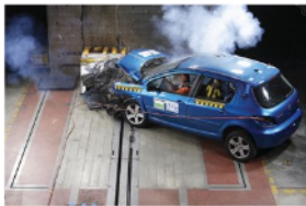
Figure 2 A crash test. Car makers test the design of a crumple zone by driving a remote control car into a brick wall.
