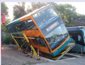
Figure 4 A toppling test
