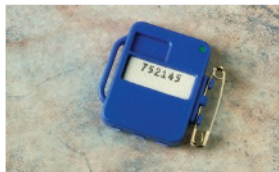
Figure 4 A film badge tells you how much ionising radiation the wearer has received. Who might wear these?
