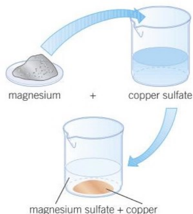
Figure 1 Magnesium displaces copper from copper(II) sulfate solution
