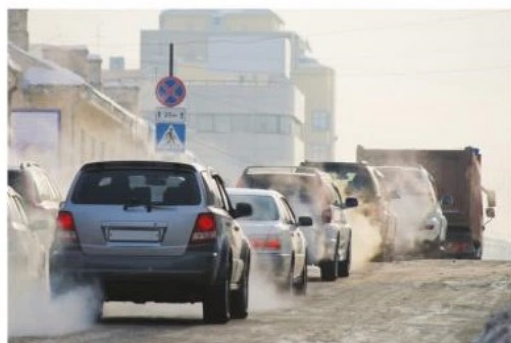
Figure 1 On a winter's day you can often see the water produced when the hydrocarbons in petrol or diesel burn, as the steam formed in combustion of the fuel condenses when it cools down
