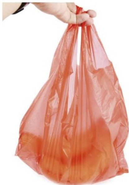
Figure 1 The forces between the molecules in poly(ethene) are relatively weak, as there are no strong covalent bonds (cross-links) between the molecules. This means that this plastic softens fairly easily when heated
