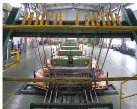
Figure 3 Drawing copper out into wires depends on being able to make the layers of metal atoms slide easily over each other, without breaking the metal
