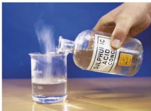
Figure 7 You should always add acid to water. Mixing acid and water is an exothermic process. If you add water to acid so much energy can be transferred that boiling acid splashes out of the mixing vessel
