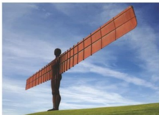
Figure 1 The Angel of the North stands 20 metres tall. It is made of steel, which contains a small amount of copper
