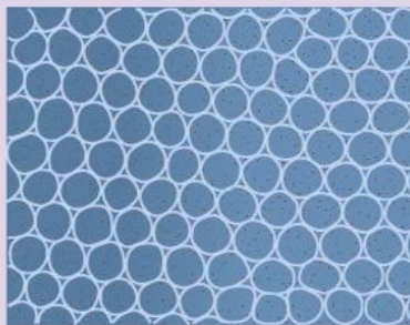
Figure 2 Making a bubble raft to model the structure of a metal
