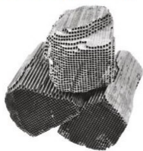
Figure 2 The transition metals platinum and palladium are used in the catalytic converters in cars. They are coated onto a honeycombed support to maximise their surface area to volume ratio
