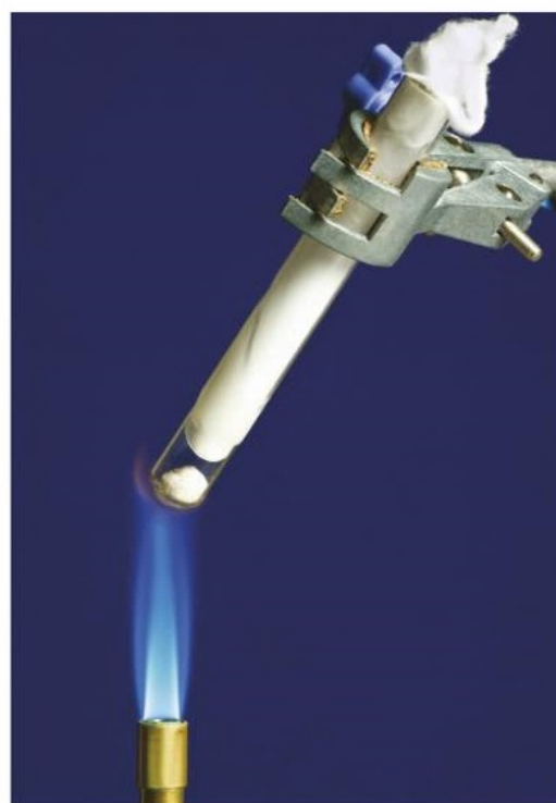
Figure 2 An example of a reversible reaction – heating ammonium chloride to break it down into ammonia gas and hydrogen chloride gas. When the gases cool down, they recombine to form the white solid ammonium chloride again
