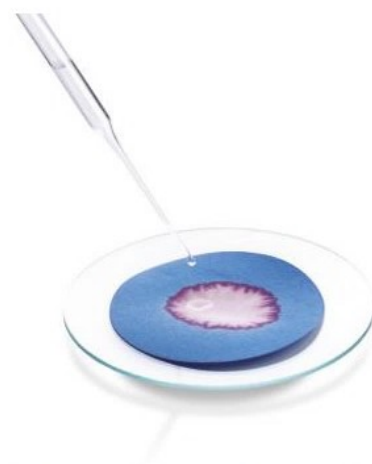
Figure 5 Blue cobalt(II) chloride paper turns pink when water is added
