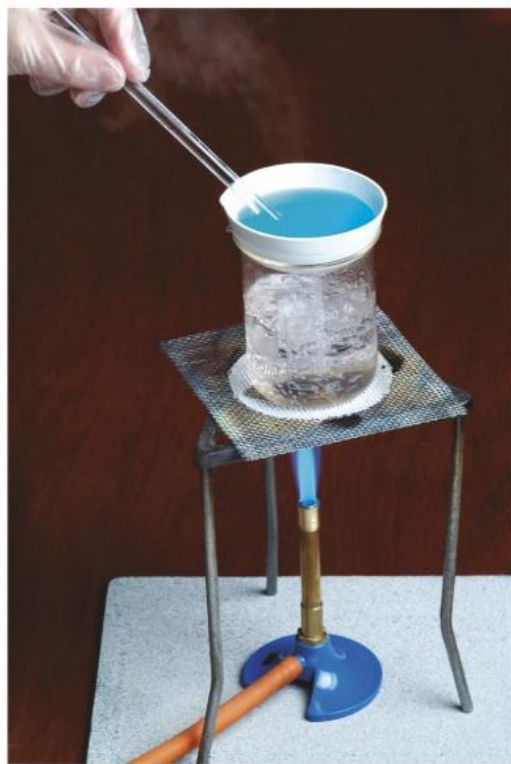
Figure 1 Heating by using a water bath is a gentler way to evaporate water from the salt solution than heating the solution directly. Steam from a beaker of water heated below the dish heats the dish and its contents. The slower the water evaporates from the solution, the larger the crystals of the salt collected at the end of the experiment
