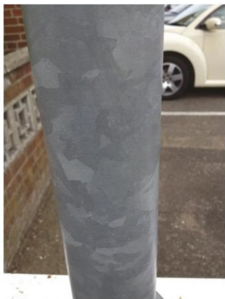
Figure 2 Metal crystals, such as the zinc ones shown on this galvanised post give us evidence that metals are made up of atoms arranged in regular patterns
