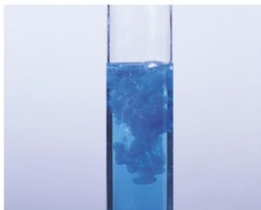
Figure 2 This distinctive blue precipitate that forms when you add sodium hydroxide solution tells you that Cu 2+ ions are present
