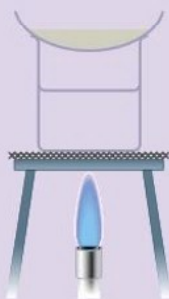
Figure 4 Evaporating ammonium sulfate solution to the point of crystallisation (when the solution becomes saturated)
