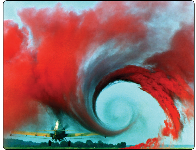
Figure 5-9. Wingtip vortex from a crop duster.
