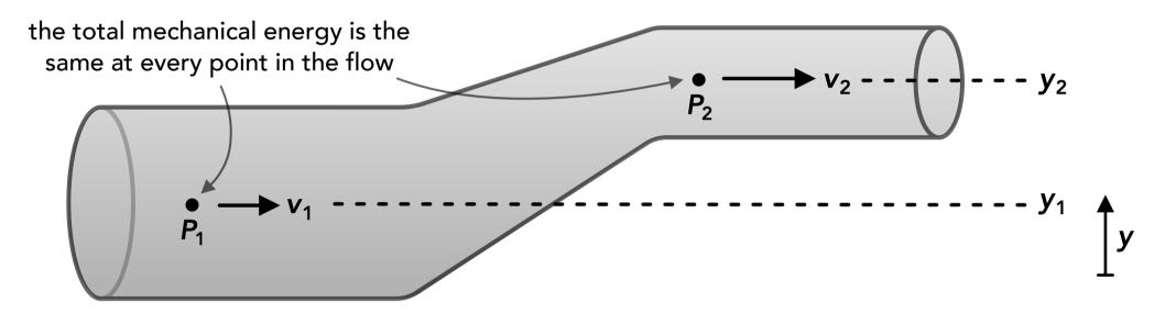
Example: What is the speed of the water at point 2? (pressures are gauge pressures)
