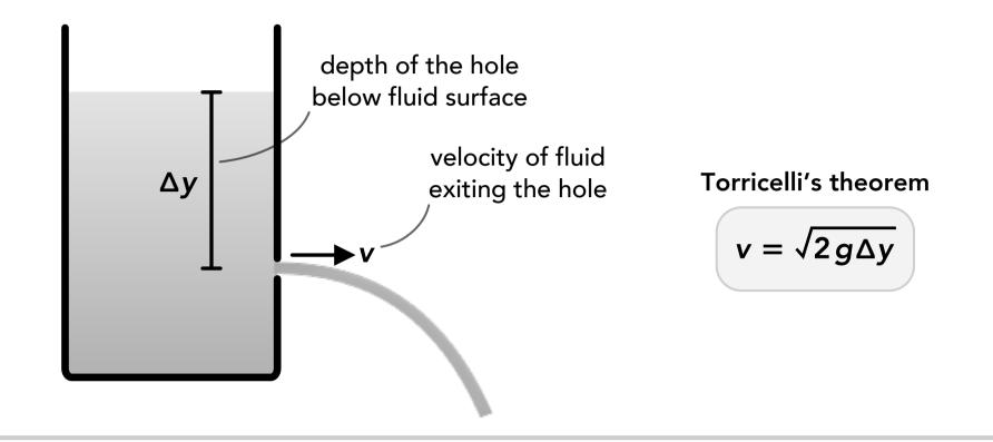
• This is just a specific application of Bernoulli's equation. We assume the velocity of the fluid at the top surface is zero, and that the fluid at the top surface and at the hole are both at the same atmospheric pressure.
