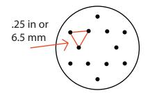
Spacing between holes doesn't have to be perfect to work, but do make sure holes are drilled perpendicular so needles won't angle towards or away from each other.
