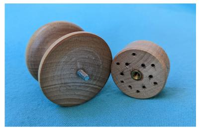
Note that no holes are drilled in the center because the threaded insert nut needs to go there, as you can see in this photo.
