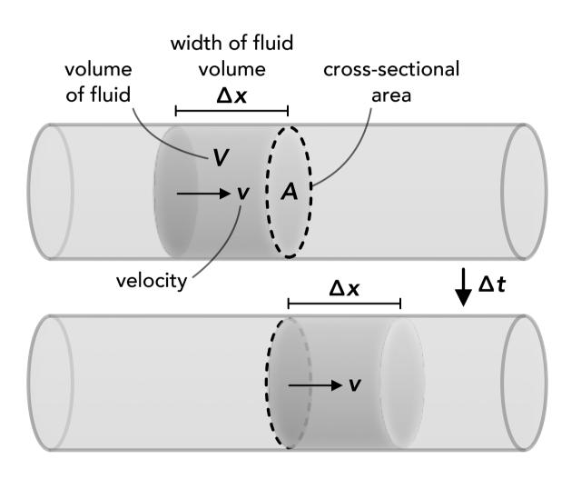
The velocity of the fluid volume is equal to its displacement divided by the period of time
