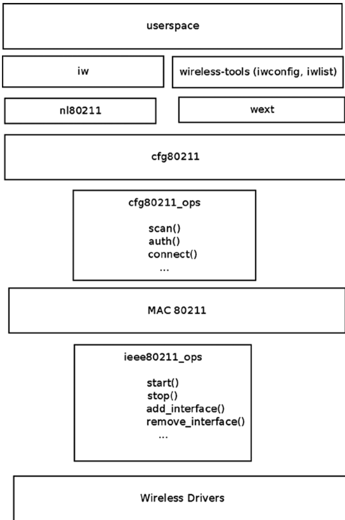
Figure 12-5. Linux wireless architecture
