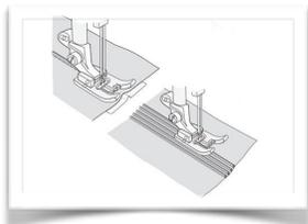
Some machines have a pintuck guide or a hole in the throat plate for this cord to run safely through.
