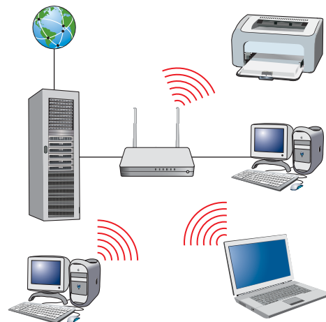
Figure 38.5 A wireless network connecting to the Internet
