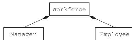
Figure 6.5 Class diagram showing composition aggregation
