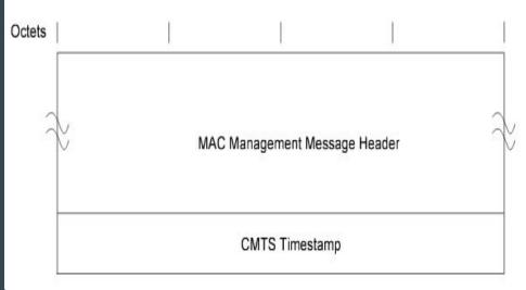
MAC Management Messages The CMTS transmits the UCD at a periodic interval to define the characteristics of a logical upstream channel as shown in the figure. The CMTS transmits a separate message for each logical upstream that is in use.
