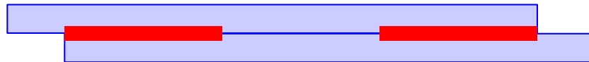
15 x bar size with 2 metal-arc fillet welds 5 x bar size in length
