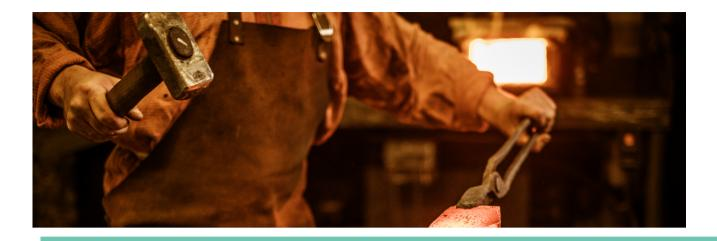
Forging- Moving metal by impact while hot. Usually with hammer and anvil.
