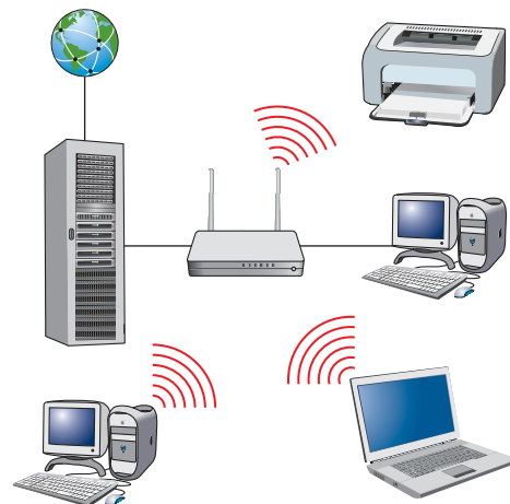
Figure 38.5 A wireless network connecting to the Internet
