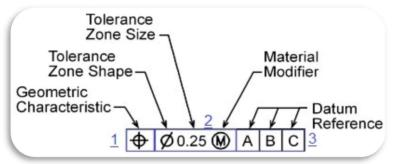
The first box or section can contain any of the 14 different standard geometric tolerance symbols found above. In this example, the feature control frame includes a True Position Tolerance.
