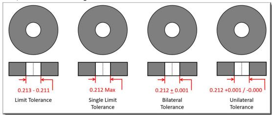
As shown, **Limit Tolerances** show both a maximum and minimum dimension allowable for the feature. A **Single Limit Tolerance** only defines one limit dimension, normally either the **maximum or minimum value** for a feature or dimension.
