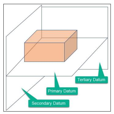
**Datums** are theoretical and only simulated by **Measurement Equipment** (Gauge pins, Granite slabs, angle plates, etc.).
