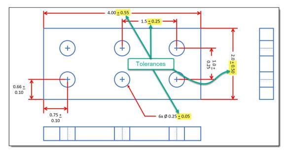
There are 4 different types of tolerances that we need to discuss, these are **bilateral tolerances**, **unilateral tolerances**, **limit tolerances & single limit tolerances**.
