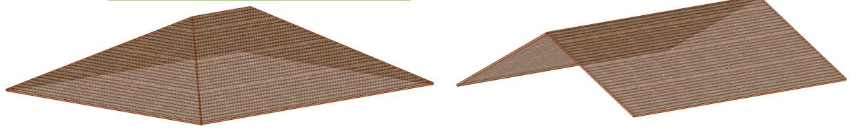
• Using Slab + Roof Element → Slab: Set Arched Slab → Roof: Adapt to Slab → delete slab entity
