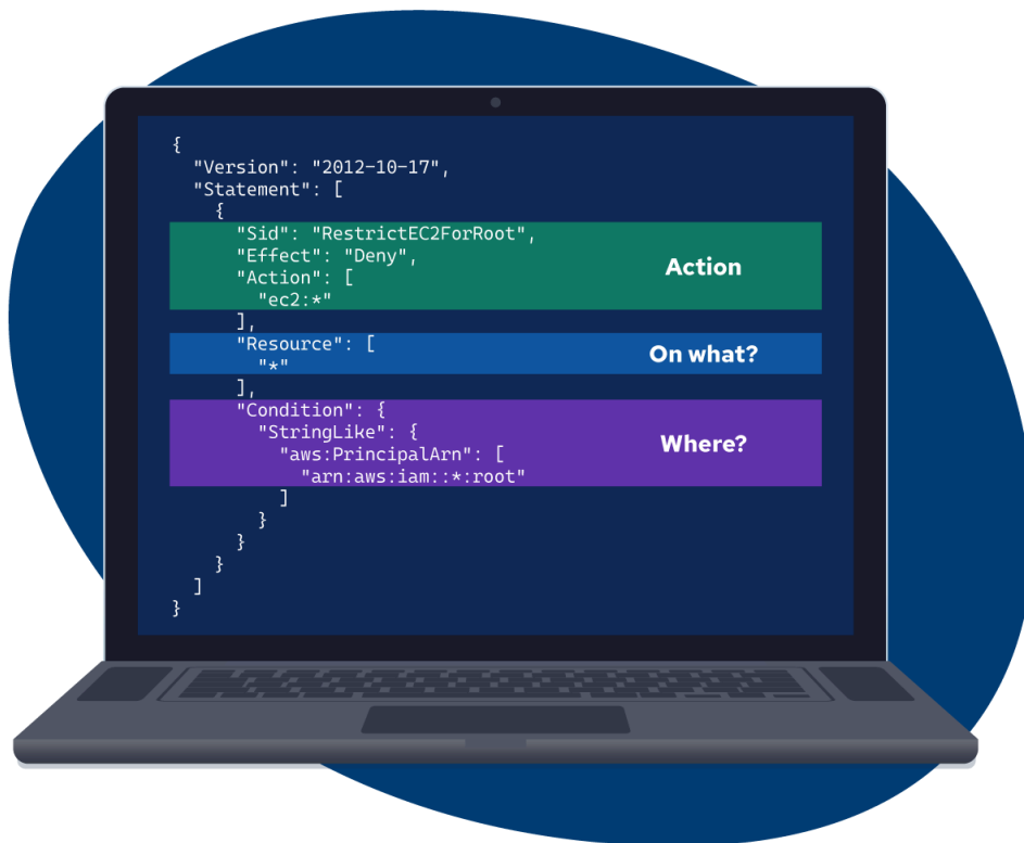
Figure 23: Example of an AWS SCP to Restrict Root User Actions
