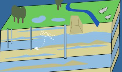
THE AQUITARD WAS DAMAGED, THERE WERE MANY OLD DISUSED BORES, PONDING OF RUNOFF FROM SHEEP PADDOCKS, AND THE AQUIFER WAS NOT HOMOGENEOUS.
