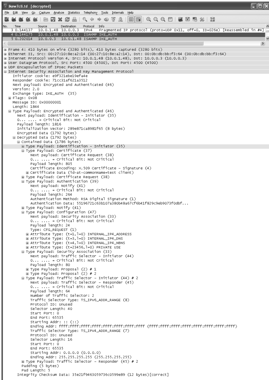
Figure 18-24 The IKE_AUTH exchange contains encrypted information and operates on UDP port 4500. The reassembly of two fragments produces an IKE message with an Encrypted/Authenticated data payload containing the following payloads: Identification initiator (IdI), Certificate (CERT), Certificate Request (CERTREQ), Authentication (AUTH), Notify (N), Configuration (CP), Security Association (SA), Traffic Selector initiator (TSi), and Traffic Selector responder (TSr).
