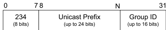
Figure 2-11 The IPv4 UBM address format. For unicast address allocations of /24 or shorter, associated multicast addresses are allocated based on a concatenation of the prefix 234/8, the assigned unicast prefix, and the multicast group ID. Allocations with shorter unicast prefixes therefore contain more unicast and multicast addresses.
