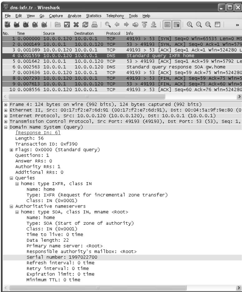
Figure 11-21 An incremental zone transfer request (IXFR record type) carried on TCP. The serial number is used to determine which records, if any, have changed since an earlier zone transfer took place.
