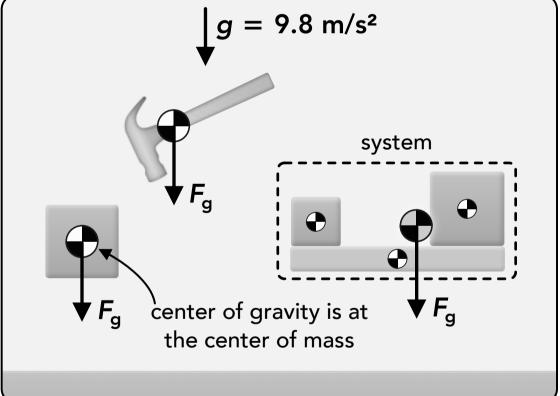
• An object or a system will balance on its center of mass (center of gravity) on a pivot point or when suspended from above. Since we can treat the individual gravitational forces acting on each object as a single gravitational force acting on the system's center of mass, that single gravitational force will not generate a torque if it's directly above or below the point of rotation.
