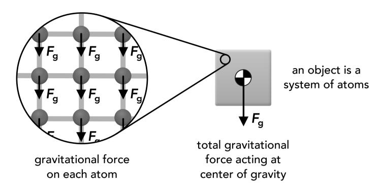
When in a uniform gravitational field, the center of gravity is located at the center of mass
