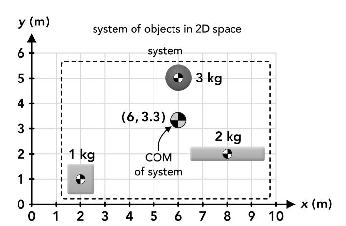
$$x_{\text{COM}} = \frac{(1 \text{ kg})(2 \text{ m}) + (2 \text{ kg})(8 \text{ m}) + (3 \text{ kg})(6 \text{ m})}{(1 \text{ kg}) + (2 \text{ kg}) + (3 \text{ kg})} = 6 \text{ m}$$
