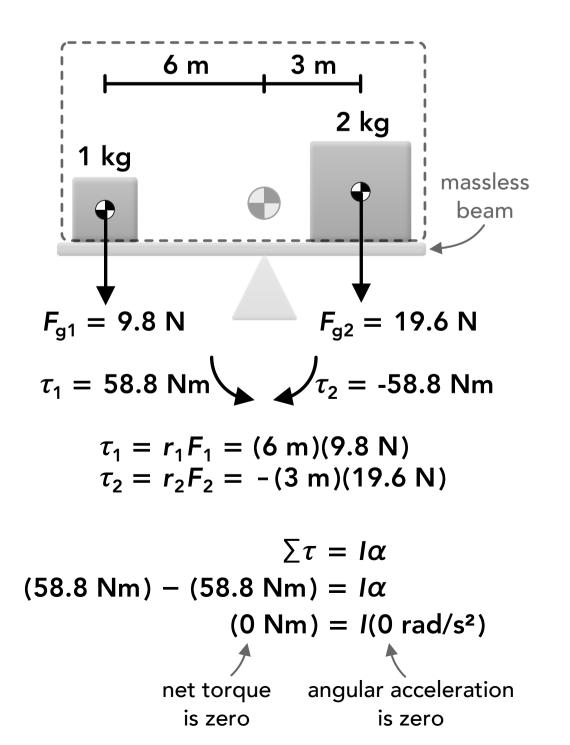
If we treat the objects as a system, a single gravitational force acts at the system's center of mass. If the pivot point is directly below the system's center of mass, that single gravitational force points directly at the point of rotation and does not generate a torque, so the net torque on the system is zero and the system is balanced.
