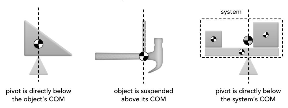
If we look at each object separately, the individual gravitational forces generate individual torques about the pivot point. If the pivot point is directly below the system's center of mass, the net torque will be zero so the system is balanced.
