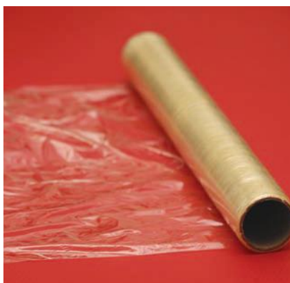
Figure 13.4 Clingfilm is just a thin film of PVC (polyvinylchloride). Its correct name is poly(chloroethene).
