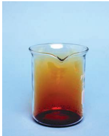
Figure 9.5 Bromine is a dark red/brown liquid – it is very volatile and gives off a toxic brown/orange vapour.
