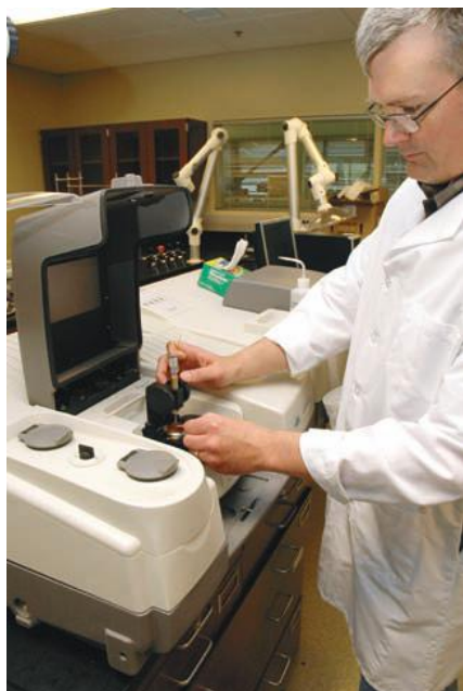
Figure 15.5 Scientists using an infrared spectrometer. The instrument covers a range of infrared wavelengths, and a detector records how strongly the sample absorbs at each wavelength. Wherever the sample absorbs, there is a dip in the intensity of the radiation transmitted, which shows up as a dip in the plot of the spectrum.
