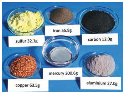
Figure 4.1 One mole amounts of copper (Cu), carbon (C), iron (Fe), aluminium (Al), mercury (Hg) and sulfur (S).
