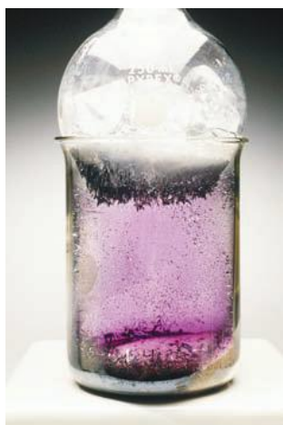
Figure 7.20 The iodine solid in the test tube has been gently heated and purple fumes of iodine gas can be seen in the inverted round bottom flask surrounding the test tube.
