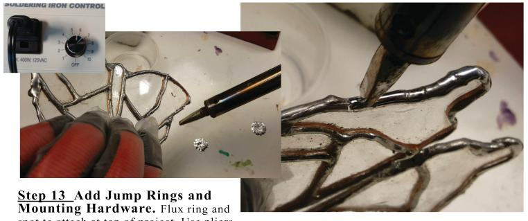
Mounting Hardware. Flux ring and spot to attach at top of project. Use pliers to hold ring. Get fresh solder dob on iron and tap melt into place.
