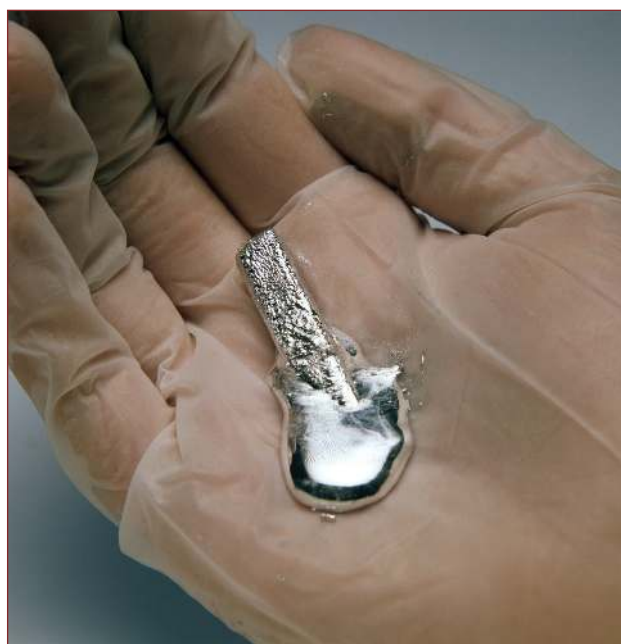
Figure 2.4 The metal gallium has a melting point just above room temperature. It will literally melt in the hand.
