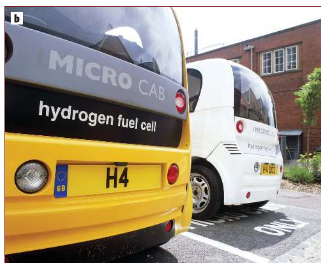
Figure 1.22 a How a car runs on a hydrogen fuel cell. The car is powered by electrons released at the negative electrode. Inside the fuel cell, hydrogen ions move to the positive electrode, where they react with oxygen to form water. b These hydrogen-powered minicabs are part of a development project at the University of Birmingham in the UK.
