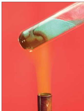
Figure 2.20 Heating copper(II) carbonate.
