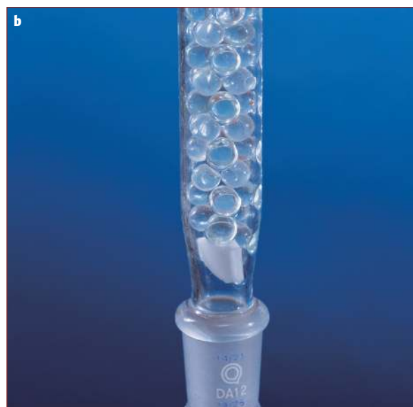
Figure 2.16 a Separating a mixture of ethanol (alcohol) and water by fractional distillation. b A close-up of the glass beads in the column.
