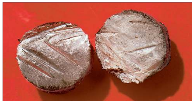
Figure 3.7 The alkali metals are all soft and can be cut with a knife. This is a sample of lithium.
