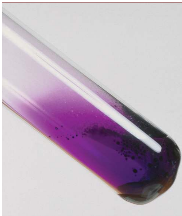
Figure 2.5 Iodine sublimes. On warming, it produces a purple vapour which then condenses again on the cool part of the tube.
