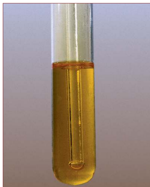
Figure 3.9 Bromine is displaced by chlorine from a colourless solution of potassium bromide.
