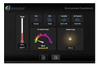
local **environmental conditions** including Ambient light, Humidity, CO2, VOCs, Air Pressure, Temperature(External Temperature probe port 1). The Dashboard also generates an Air Quality value by combing the CO2 and VOC values.
