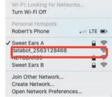
The ID number in the "System Check" is your databot™'s unique identification number! Now, disconnect from System Check, turn off databot™, and turn it back on in Server Mode. The green indicator light will be pulsing and databot™ will be broadcasting its unique ID number. Connect to it like any network.
