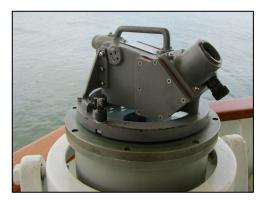
The telescopic alidade is made to fit over the gyro compass repeaters on the bridge and is used to quickly and accurately measure the true bearing to any object.
