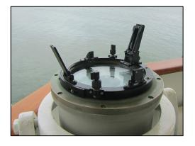
obtain a highly accurate bearing. It is most often used in gyroscopic error by azimuth calculations. This topic is covered in chapter 9 and 10 of this text.
