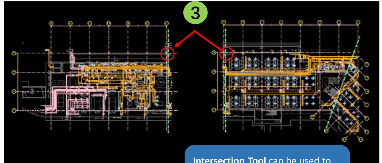
**Intersection Tool** can be used to accurately move drawing to intersection point
