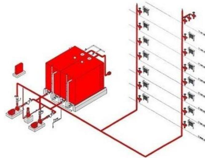
Typical Arrangement of Wet Riser System
