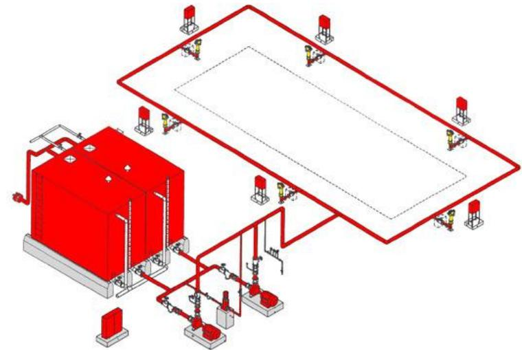
Typical Arrangement of Hydrant System
