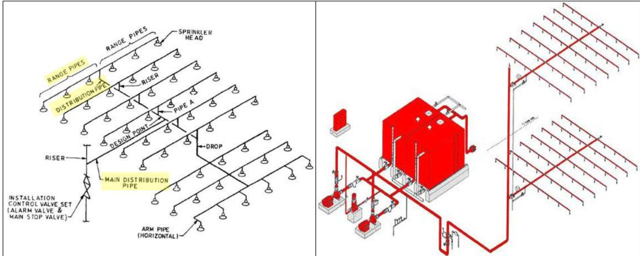
Typical Arrangement of Sprinkler System
