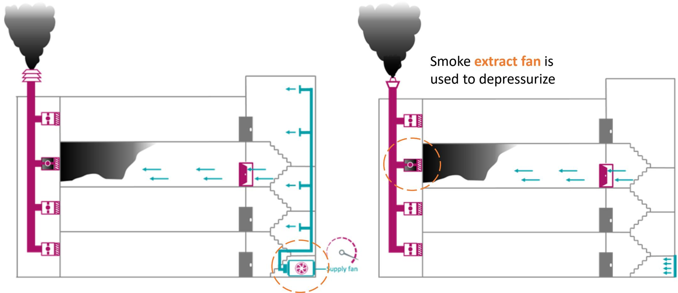
A pressurisation **supply fan** is used to pressurize the protected space
