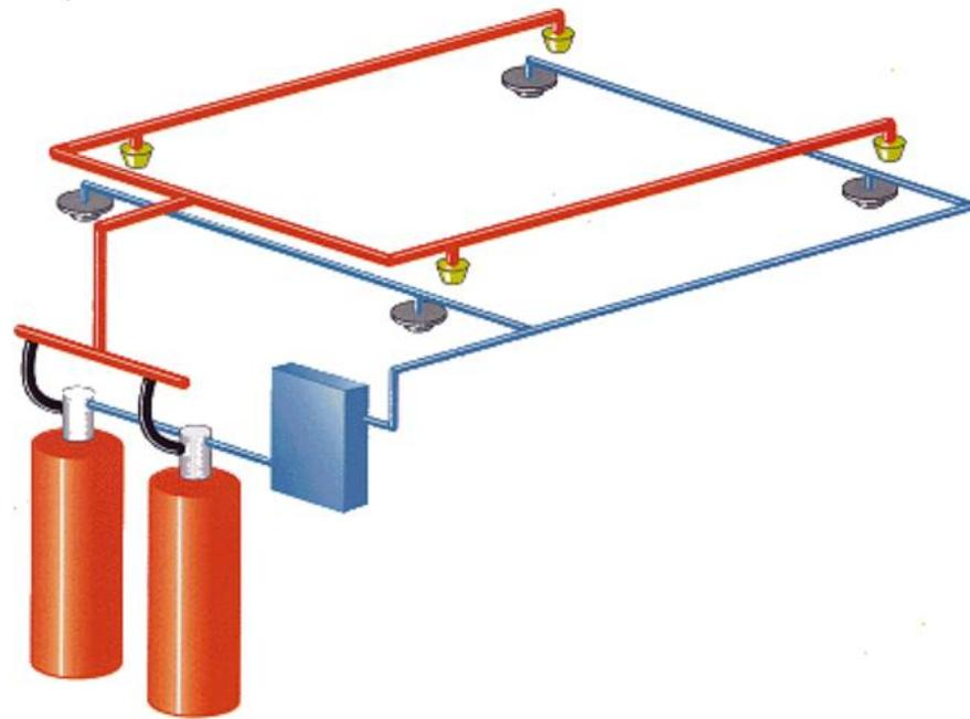
Typical Arrangement of Gas Suppression System
