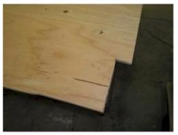
You need to notch out the plywood, so that the shelf will fit around the legs of the worktable. It's a good idea to install it before the top goes on.
