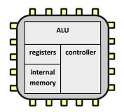
The **CPU** (**Central Processing Unit**) is the main component in a computer for processing data and instructions. It could be considered as the computing equivalent of the human brain. It is a hardware device that is made up of many sub components:
