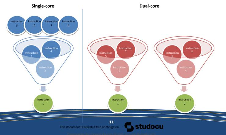
In a single-core CPU each instruction is processed one after the other, whereas in a dual-core CPU, two instructions may be processed at the same time. In theory, a dual-core CPU should be able to process instructions twice as fast as a single-core CPU. However, this isn't always the case as sometimes *Instruction 2* may need the result of *Instruction 1* before it can be processed.
