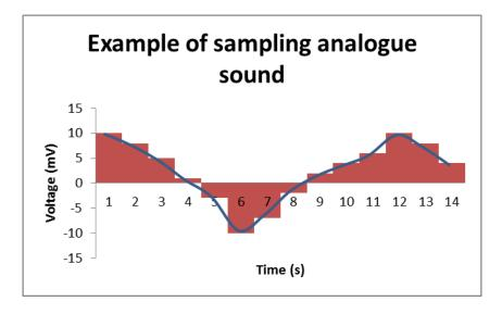
The number of times that the sound level is sampled per second is called the *sampling frequency*. The higher the sampling frequency, the better the quality of the sound recorded. A typical sampling frequency is 44,000 times per second, also known as 44 kHz. This is the sampling frequency used on most audio CDs.
