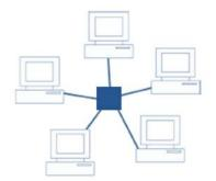
In a star network, each computer system is connected to a central node, also known as a hub.
