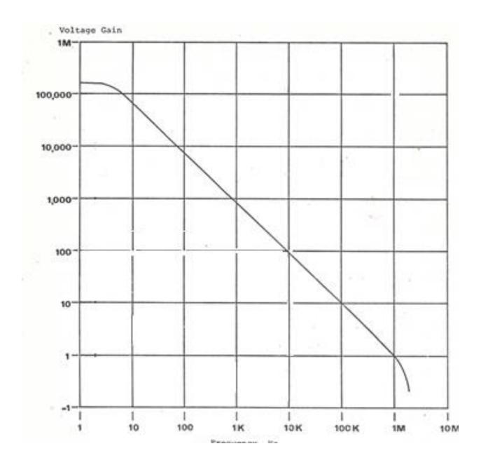
From the Graph above: Circuit designer has designed a circuit that has gain of 50 he believe's that operational amplifier with a constant gain to a frequency 100 Khz. Will this work using the graph at top? No
