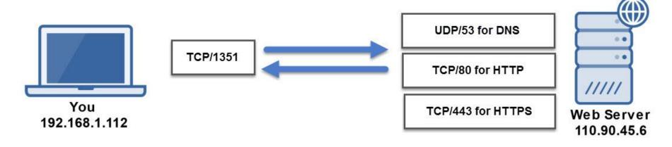
Communication originates from your computer utilizing a **high random port** to communicate across a LAN / WAN / Internet to communicate with a remote server, in this case a web server. The Web server will be listening in on specific ports for its associated TCP/IP protocols.
