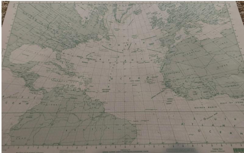
Step 1: Plot the origin and arrival positions on the tracking chart and draw the trackline.
