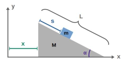
Hint: The Lagrangian for the system consists of the kinetic and potential energies of both the ramp and the block. Since the ramp is fixed at the y = 0 level, its potential energy is zero. You need to find the kinetic energy of the ramp well as the kinetic and potential energy of the block and express these in terms of x and s.
