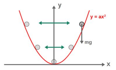
In this problem, you have one object in two dimensions with one additional constraint (the particle must stay on the parabola), so you need  $1 \cdot 2 - 1 = 1$  generalized coordinate to describe the system with.
