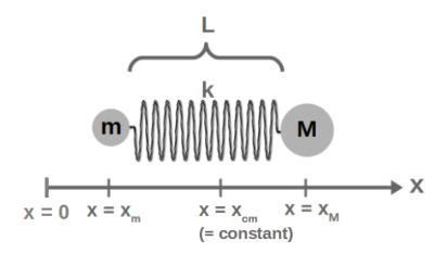
The spring is then stretched from equilibrium by an amount  $\delta$ , so that it begins oscillating. As the spring oscillates, the displacement  $\delta$  changes with time, so  $\delta = \delta(t)$ .
