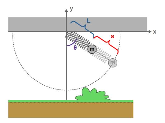
**Find the Lagrangian and the equations of motion** for the pendulum bob using the above mentioned generalized coordinates. Check that the equations of motion reduce to those of the simple pendulum in the limit that the spring constant  $k \to \infty$  (in other words, the spring becomes completely rigid).
