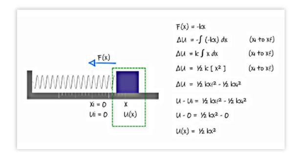
By setting the reference potential energy  $(U_i)$  to zero when the spring is at its relaxed length  $(x_i = 0)$ , we obtain the formula for the elastic potential energy at any position x:
