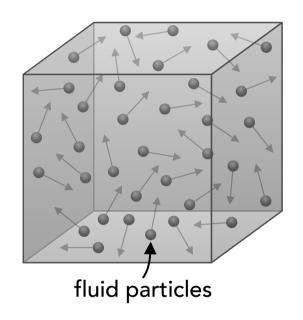
fluid particles move randomly, colliding with other fluid particles and the container walls
