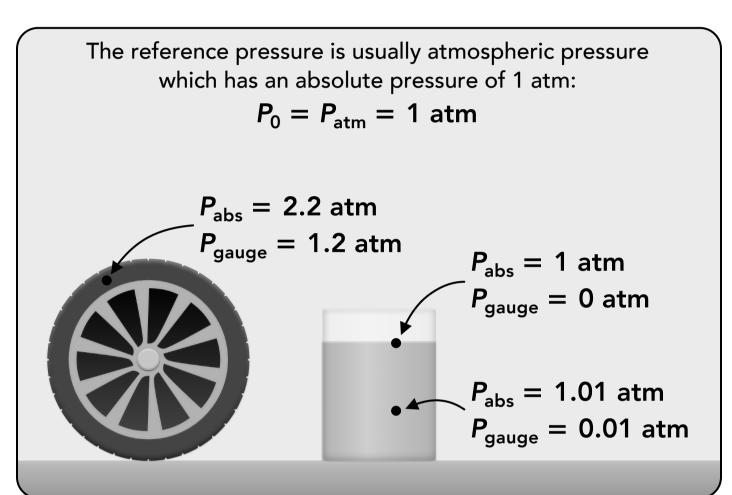
• The word "vacuum" is sometimes used to describe a gauge vacuum, which is when the gauge pressure is negative (the pressure is lower than the atmospheric pressure or reference pressure, see the diagram above). So it's important to be clear about the difference between "absolute/perfect vacuum" and "gauge vacuum".
