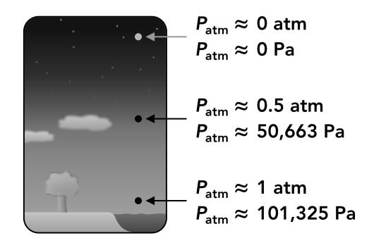
Any liquid surface that is exposed to the atmosphere will be at atmospheric pressure (1 atm)
