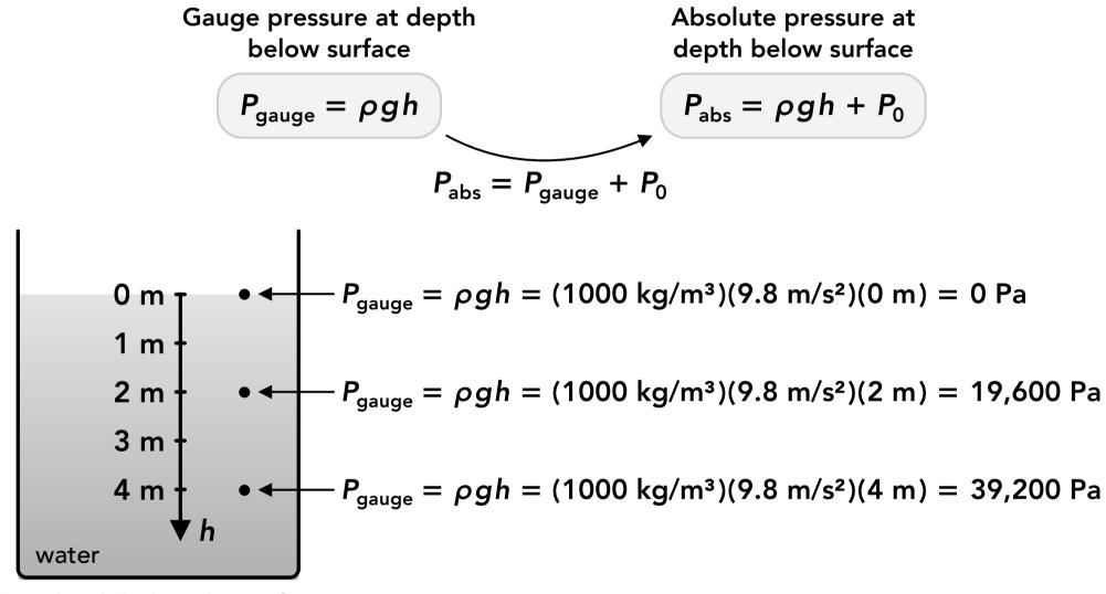
h is depth below the surface of the fluid, down is positive
