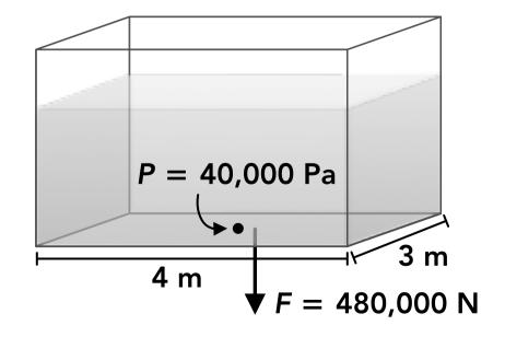
$$P = \frac{F}{A} \rightarrow 40,000 \text{ Pa} = \frac{480,000 \text{ N}}{(4 \text{ m} \times 3 \text{ m})}$$
